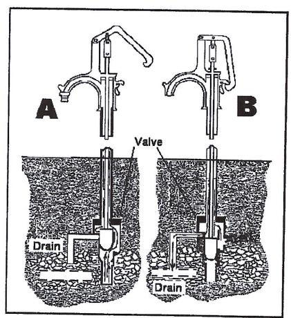
Because the drain port is open when the hydrant is in the off position, it provides a **convenient route through which impure groundwater**, **insects and dirt can enter the hydrant**, thereby contaminating the water supply. Regardless of whether the hydrant is in the on or off position, contamination of the hydrant and water distribution system is possible under a variety of circumstances.
